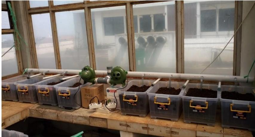
**Gambar 3.** Reaktor *static aerated biopile*
